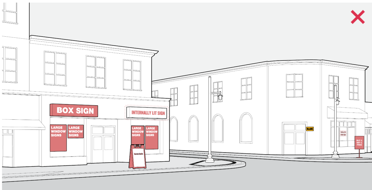
Figure 34: Prohibited Sign Designs - Illustration of prohibited signs in pedestrian-centric areas, including internally luminated signs, simulated neon signs, box signs, and molded plastic A-frame signs.
