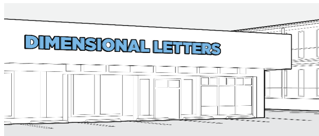
Figure 43: Individual letters mounted directly on the building are recommended, especially where the building has a sign fascia.
